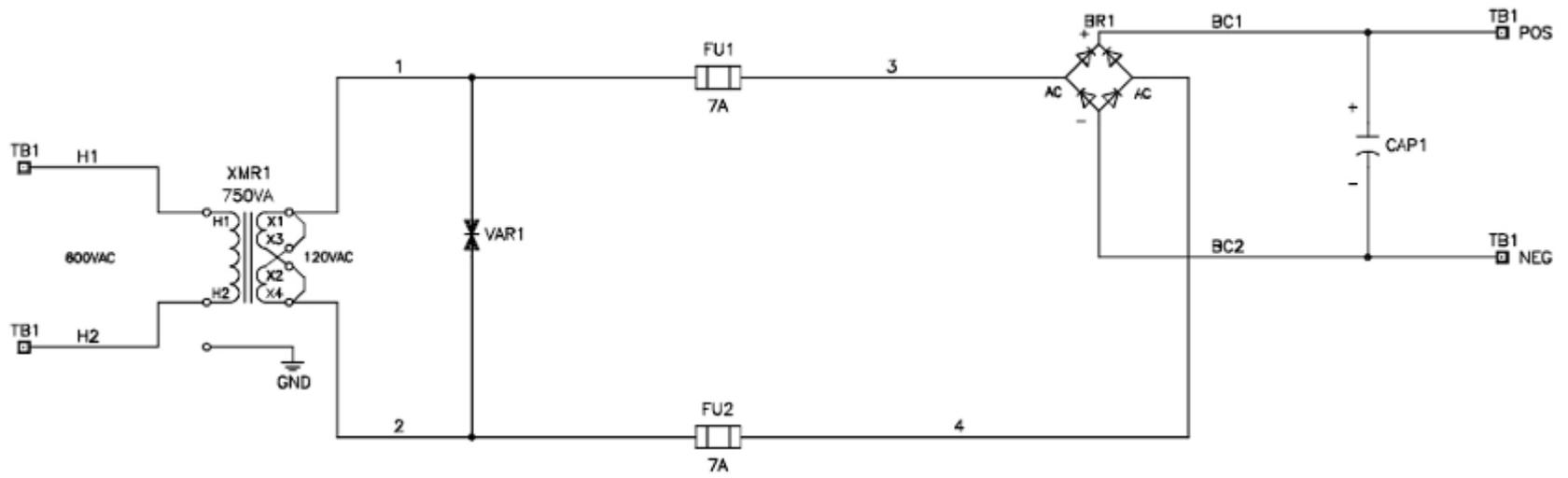
**Figure 2: Brake Rectifier Schematic (Single Brake Coil)**
