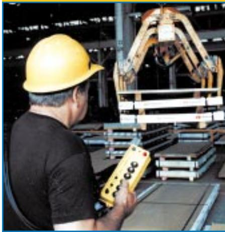
Martin Kaminski uses Telemotive’s 10-K pendant style radio transmitter, which plays an integral part in Ryerson’s overall productivity.
